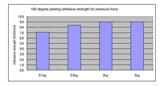
●180 degree peeling adhesive strength – variation after applying
